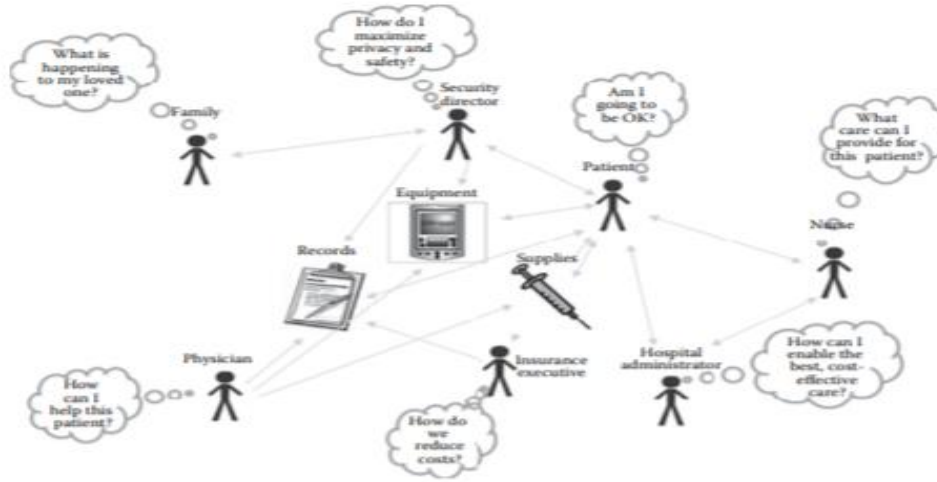
Figure 2.5 First iteration rich picture for a healthcare IoT system. (Adapted from Laplante, N.L., et al., IEEE Syst. J. , 2016.)
